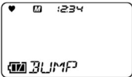
The LCD display shows a battery icon, a heart icon, a square icon, and the number 1234 at the top. Below this, the word "BUMP" is displayed in a large, pixelated font.         | S. 41         |
